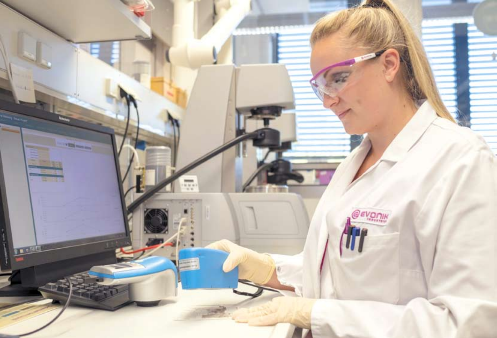
Katrin Basler (chemical laboratory assistant at Evonik Oxeno) checks the yellowness-index of a weathering sample of a PVC roofing membrane that has been exposed for 24 months.
